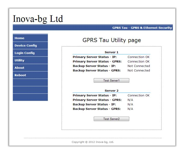
In **Utility** menu, connections to the servers can be tested. When the test button is clicked the device will send test messages by IP and/or GPRS to the server, corresponding to the mode selected for the server. If a backup server is enabled – the device will test this connection also.
