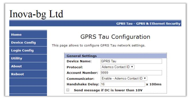
**Device Name** – Enter the name of the device. This value is used only for user convenience – to identify devices if you have more than one connected to one network. Maximum length – 30 symbols.
